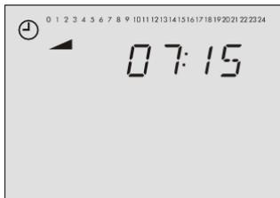
1. Turn the rotary switch to (controller time). Display: time, and blink.
