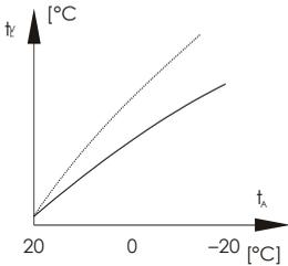
The gradient needs to be increased **if the room temperature drops when it is cold outside.**
