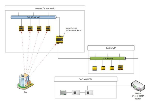
Figure 3 Various BACnet networks and devices
