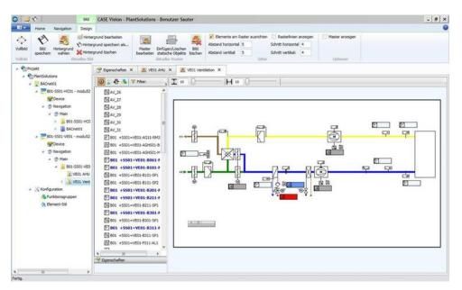
The CASE Vision program is designed for the simple creation of **system navigation trees** and **dynamic** system diagrams for various visualisation applications from SAUTER.
