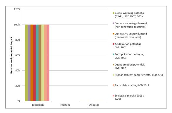
The valve is used as a control element in combination with an actuator. The present eco-balance describes the ecological impact of the production and the disposal of the valve. The environmental impact of the actuator, including its energy requirement, is measured and evaluated separately.
